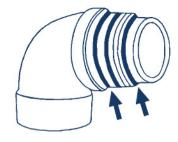
Install the new O rings on the sleeve, dust seal to the rear, product (pressure) seal up front.
