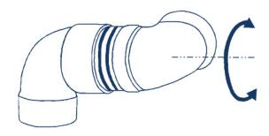
Insert the sleeve into the body, slowly rotate the sleeve while inserting into the body.
