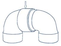
Reinstall ball retainer screws until tight. If this interferes with the smooth rotation of the ball bearings, then back off 1/8 - 1/4 turn. A thread locking sealant is recommended to prevent screws from backing off. After pressure testing, the unit is ready for installation.
