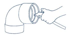
Remove the ball retainer screws. Add a sufficient amount of solvent into each raceway to flush out the lubricant. Rotate the sleeve, catching the balls as they fall out. When all the balls have been removed, the body and sleeve can be separated. Discard old seals. Thoroughly clean the body and sleeve.
