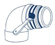
Lubricate the body and the sleeve with grease.
