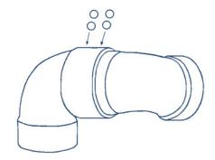
When the sleeve is fully inserted, feed the ball bearings into the raceways while rotating the sleeve. To make space for all the balls, insert a screw driver into the raceway, while continuing to rotate the sleeve in one direction (be careful not to damage the threads). This will cause the balls to jam up, making room for the remaining balls. Now reverse rotation of sleeve and insert the remaining balls.
