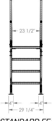
STANDARD FEATURES MODEL NUMBER: COL-4-36-23 **OVERALL SIZE:** 29 1/4" W x 79" L x 82 7/8" H **CLEARANCE SPAN:** 26 1/8" W x 38 1/4" H TOP PLATFORM HEIGHT: 40" STEP HEIGHT SPACING: 10" STEP DEPTH: 7" STEP & PLATFORM WIDTH 23 1/2" CLIMB ANGLE: 58° **ALL STEPS & PLATFORM ARE** SERRATED STEEL **KNOCK-DOWN HANDRAILING** (UNIT SHIPS KNOCKED DOWN, ASSEMBLY REQUIRED)
