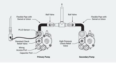
Manifolded systems provide up to 2X the flow rate and improved uptime. Manifolded systems can be configured in sumps 42" in diameter or greater.
