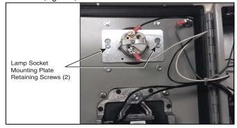
Figure 2. Remove Lamp Socket
