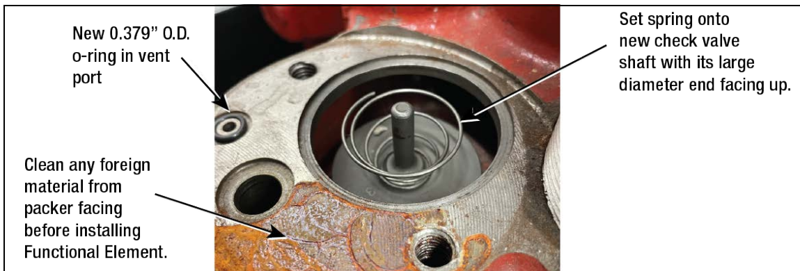
Figure 10. Installing Check Valve And Spring In Packer
