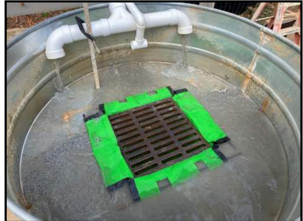
Product Installed / Grate In Place / Test Initiated
