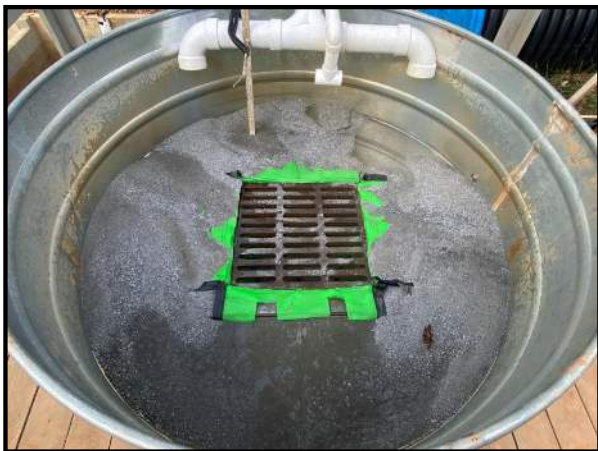
Deposition At End-of-Test / Close-up of Captured Sediment
