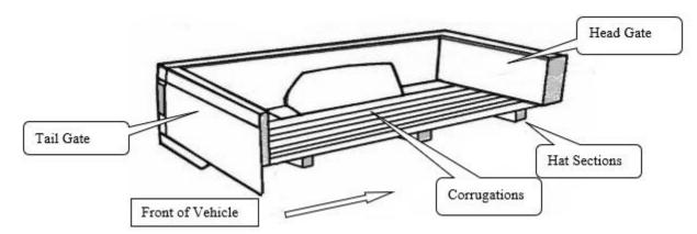
Figure 1: This cutaway drawing shows the head gate and bed corrugations.
