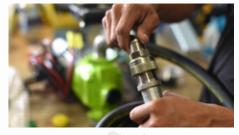
**7.** Connect swivel to opposite end of the hose using provided Teflon tape.
