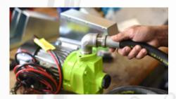
**6.** Connect hose to elbow using provided Teflon tape.
