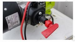
**10.** Use provided key (in red) to turn pump ON/OFF as needed.
