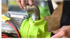
**5.** Screw elbow into top of pump opening using provided Teflon tape.
