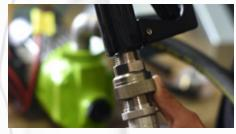
**9.** Attach swivel (and hose) to nozzle using provided Teflon tape.
