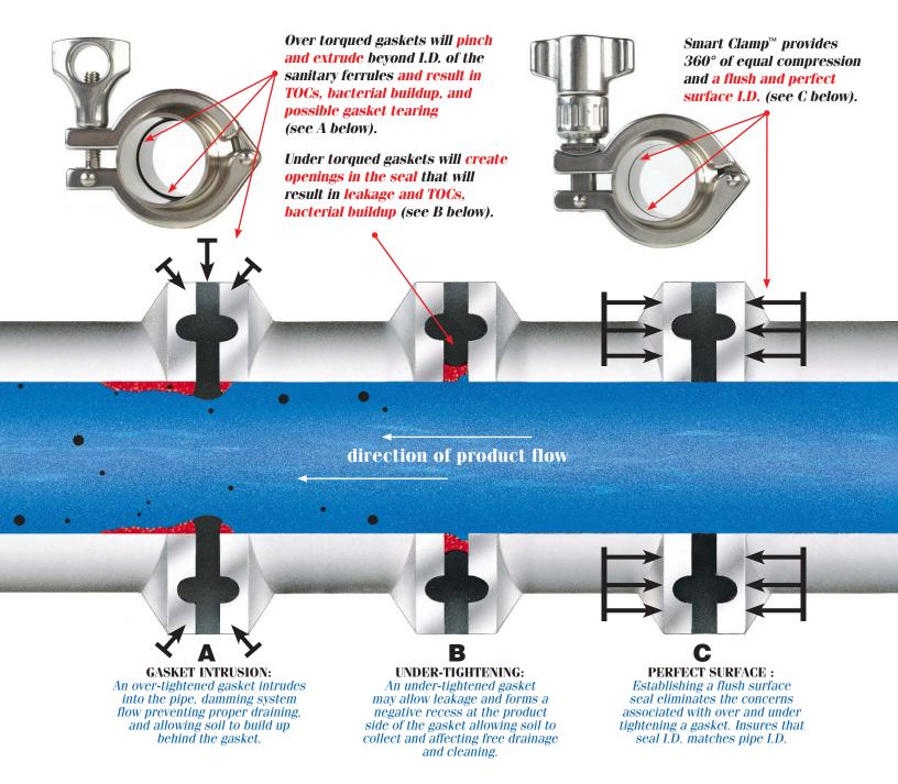
When a gasket is under-tightened, the result is a negative recess between the ferrules allowing soil and bacteria to accumulate and become entrapped (see B in illustration).
