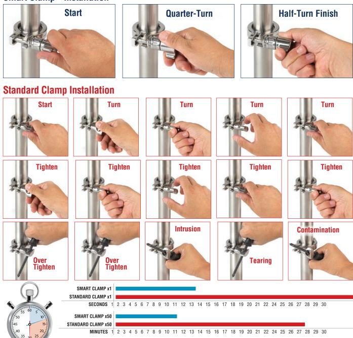
Time is based on typical gasket change out. Time is to open clamp, change out gasket, and close clamp. For this demonstration, ten seconds are included to each gasket change out. Smart Clamp may not be effective in severely worn or pitted ferrules or with severely degraded gaskets
