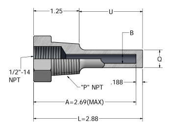
Material: 316 Stainless (std) Dimensions (inches): Bore Dia. B: .260" bore, for 1/4" dia. Element" Element Length A: 2.5" Overall Length L: 2.88" Insertion Length U: 1.63" Process P: 1/2" NPT .500" Shank dia. Q:
