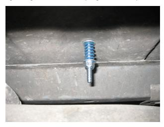
This spring bolt combination will anchor the tank while still allowing the tank to move with the bed of the truck as it travels over rough terrain. This will prevent undue stresses from being passed along to the tank from the truck.
