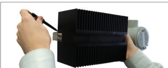
Figure 5 – Scribe the side of the mounting bracket
