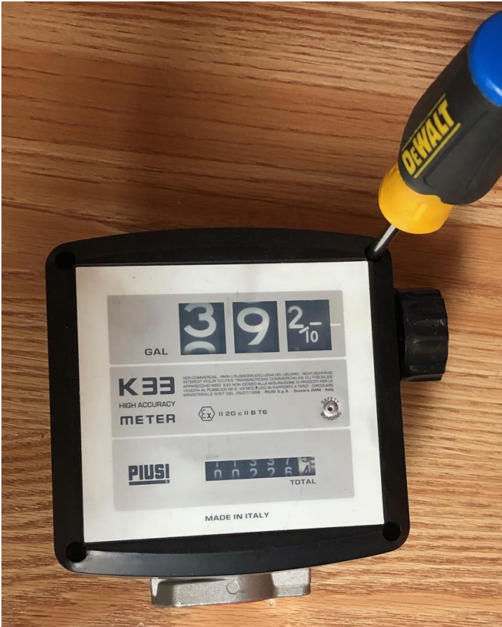
Step 1: Remove four screws from meter face cover
