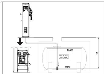
DIAGRAM: FIXING THE UNIT TO THE GROUND
