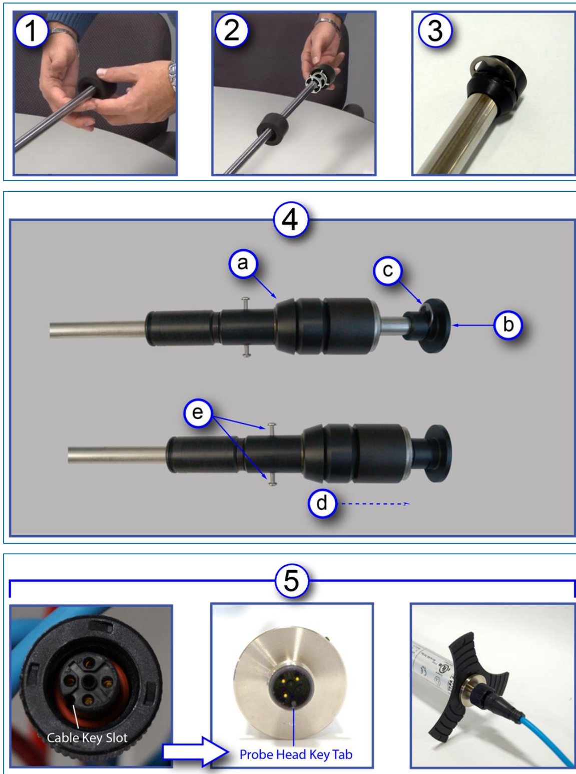
Figure - 3 Level Indicator, AEF and Cable Installation
