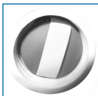
Figure 9-1 Sensor with Belcor® Carbon/polymer Strip
