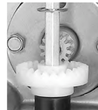
Adjuster drive gear engaged at bottom
