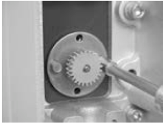
Remove Packing Gland Mounting Screws
