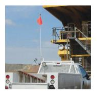
FS5X-O General-Purpose Warning Whip, non-lighted, 5 ft with hex base, 12" orange flag with white reflective X Att General Purpose Warning Whip, lighted, 5 ft with hex base, FS5XI-O 12" orange flag with white reflective X △++ FS8X-O General Purpose Warning Whip, non-lighted, 8 ft with hex
