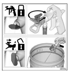
Engage Trigger Lock. Rotate Spray Tip back to SPRAY position. Disengage Trigger Lock and continue spraying.
