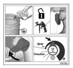
9. Continue triggering Spray Gun into waste bucket for 1 to 3 minutes.
