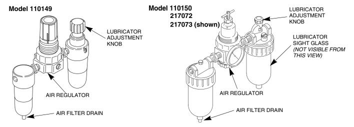
Before installing any air line components, blow out the pipe line to remove scale and other debris. Use pipe compound or tape sparingly and only on male threads.
