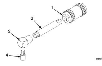
360° Grease Swivel & Coupler Kit 203597 6000 psi (420 bar) Maximum Working Pressure
