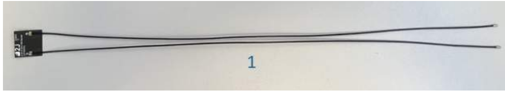
Figure 4-43 - Wi-Fi + BT Modem Module Assembly Parts
