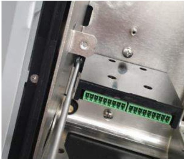
Figure 4-17 - Fastening Point of the Electronic Pump Module on the Left
