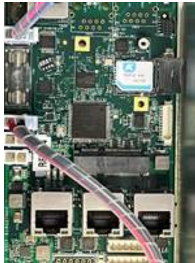
Figure 4-35 - microSIM on SIM Socket
