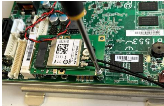
Figure 4-53 - Modem Assembly on the mPCIe Connector
