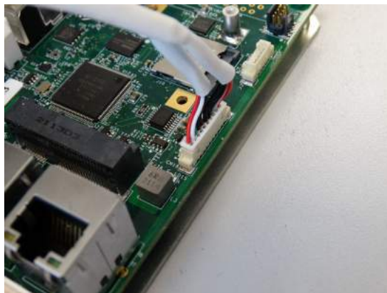
Figure 4-41 - USB Installed on CommBoard
