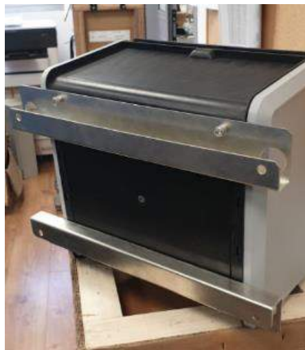
Figure 4-4 - Site PRIME with Rails Installed
