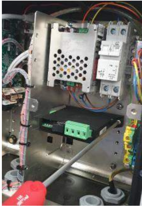
Figure 4-16 - Fastening Point of the Mechanical Pump Module on the Right
