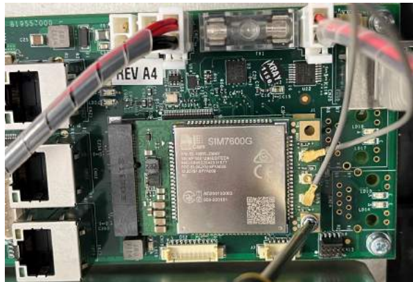
Figure 4-40 - Module on the CommBoard mPCIe Connector
