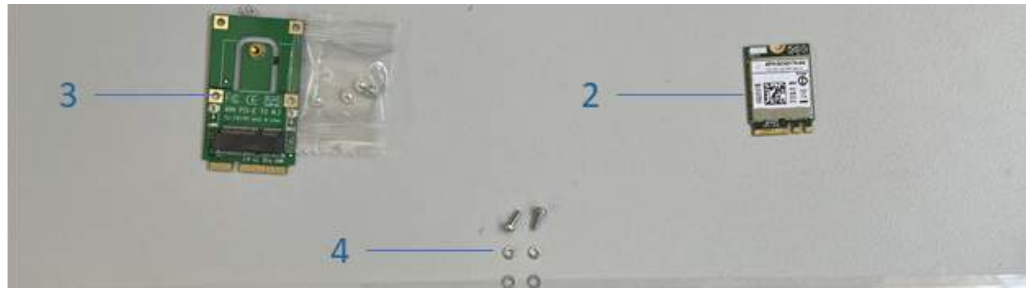
Figure 4-44 - Wi-Fi + BT Modem Module Assembly Parts
