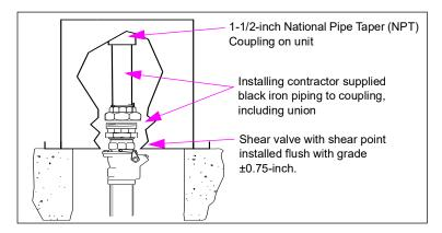
Follow shear valve manufacturer's instructions for installation procedures, testing, and other procedures.
