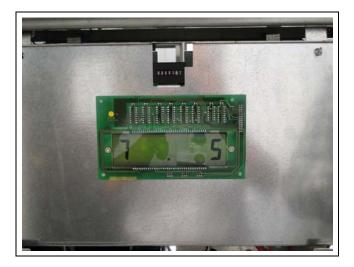
2 After the required can size is displayed, remove the nozzle and switch on the pump handle. This selects the can size for calibration.
