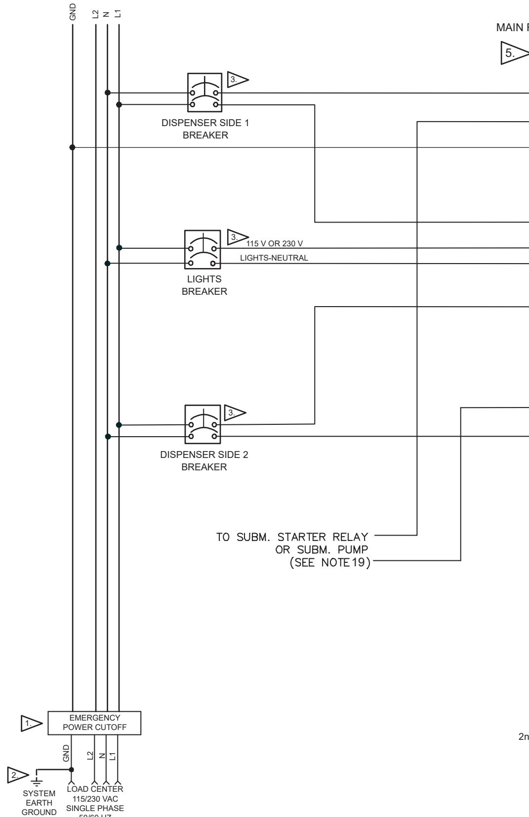
NOTE: Dual-sided unit shown. For single-sided unit make side 1 connections and cap side 2 wiring. All unused wiring must be capped properly.
