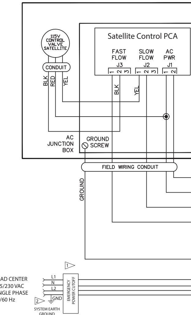
**NOTES:** 1. Dual sided unit shown. For single-sided unit make Side 1 connections and cap Side 2 wiring. All unused wiring must be properly capped.
