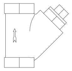
THE STRAINER SHOULD BE PLACED IN-LINE AT THE INLET OF THE DISPENSER, BETWEEN THE DISPENSER AND THE EMERGENCY SHUT-OFF.
