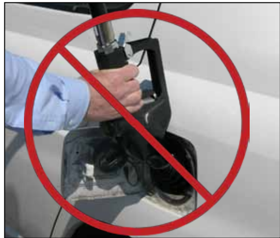
Figure 2: Wrong Nozzle Position
