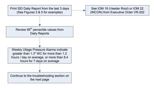
When responding to Weekly Ullage Pressure Alarms the following procedure shall be followed:
