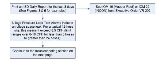
When responding to Ullage Pressure Leak Test Alarms the following procedure shall be followed:
