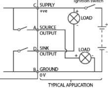
NOTE: IF SINK ONLY OUTPUT IS REQUIRED THEN PIN A IS NOT USED.
