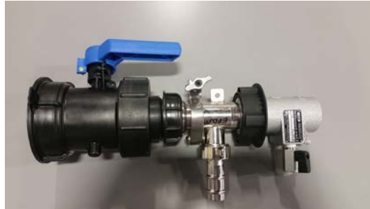
100mm Buttress IBC Connection
