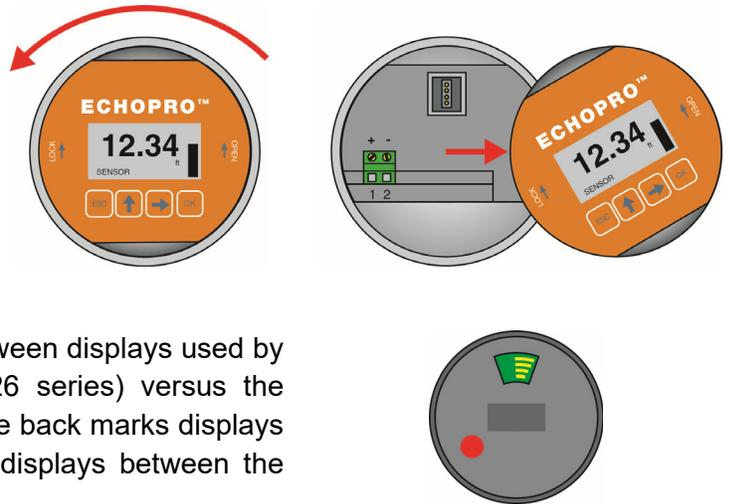
**Note:** There is an internal configuration difference between displays used by the EchoPro® sensors (LR11, LR16, LR21 and LR26 series) versus the display used with the LR98 series. A colored dot on the back marks displays to be used only with the LR98 series. Never swap displays between the LR98 series and other EchoPro® sensors.
