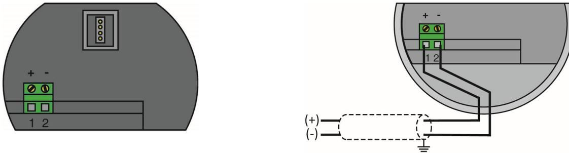
The sensor should be wired with shielded 2-conductor cable (16 to 22 AWG) to protect from electromagnetic interference. If using a liquid tight connector, select a cable with an outer diameter that is designed to ensure an effective seal with the connector [typically between 0.20" to 0.35" (5 to 9 mm)].
