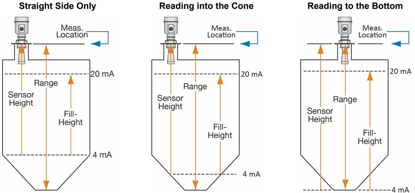
The location of the sensor is not critical because the lowest level reading is within the straight side of the tank.
