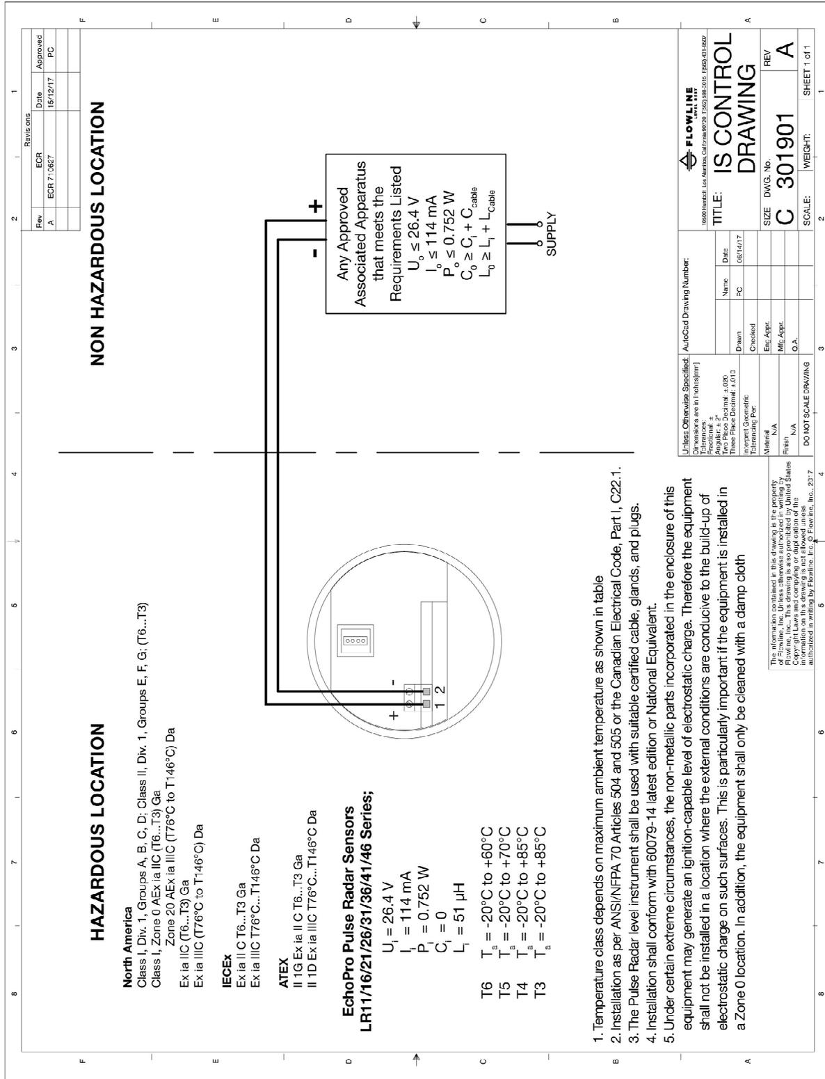
The cabling should be a shielded twisted pair to minimize EMI interference. Typically 20 to 24 gauge wire is used in this application.
