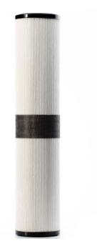
Facet FA Series microfilters offer superior filtration for removing ultra-fine solid contaminants such as rust, scale, granular and other types of solids from aviation fuel systems. They are designed to flow from the outside to inside.
