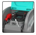
**3)** Remove fill cap and put fuel in unit through fill port.
