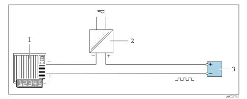
1 Automation system with pulse output and frequency input, e.g. PLC
