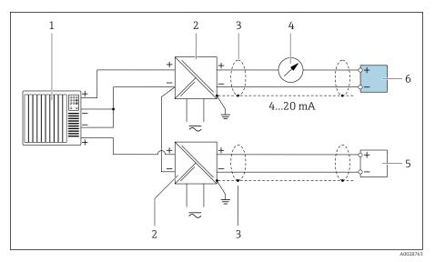
**E** 1 Connection example for HART input with a common negative (passive)
