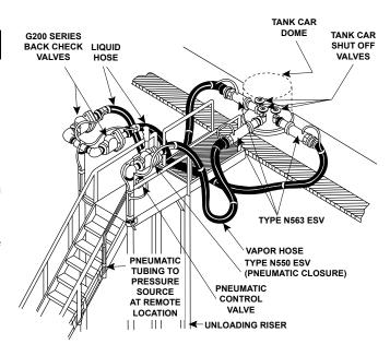
Figure 2. Typical Railcar Hook-up
