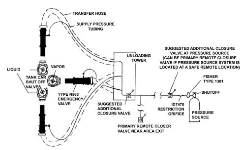
Figure 3. Installation Schematic of N563 Series
