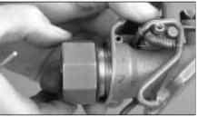
6. Insert the swivel into the coupler body until it is fully seated. A slight rotation assists with this assembly.
