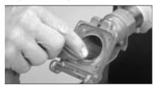
1. Clean the body fully in the disc stem hole and the stem seal areas. Check for any corrosion, gauling or damage to the body in these areas.
