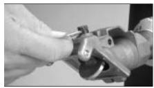
2. With the disc rotated a half turn or 180° from the closed position, remove the disc retaining pin from the top of the disc stem. If necessary, use a hammer and lightly tap the pin out.
