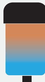
An orange color indicates the silica gel has absorbed oil and moisture.
