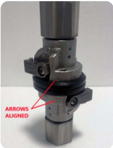
03 While continuing to push the parts together, twist the two couplings until the arrows align. The parts will “click” when fully engaged.
