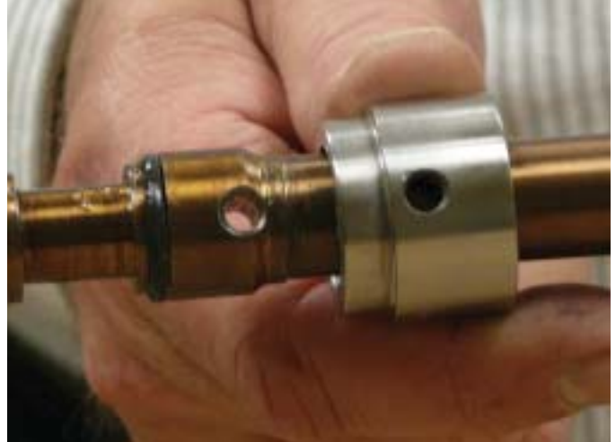
Figure 9-19 Align Spirol Pin Hole on O-ring Sleeve with Matching Hole on Shaft
