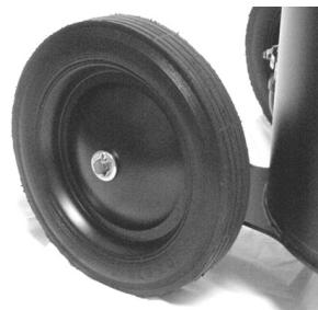
3. Install front casters by inserting bolts up through caster and weldment then secure with nuts provided.
