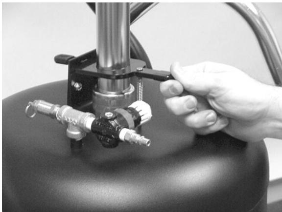
When the bowl is at the desired position, release the locking bar to secure the bowl and drain pipe in place.
