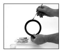
**CHECK & LUBRICATE GASKET—** Check gasket to be sure it is compatible for the intended service. Apply a thin coating of Gruvlok lubricant to the exterior surface and sealing lips of the gasket. Be careful that foreign particles do not adhere to lubricated surfaces.
