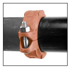
ASSEMBLY IS COMPLETE— Visually inspect the pipe joint to assure the coupling keys are fully engaged in the pipe grooves and the bolt pads are in firm even metalto-metal contact on both sides of the coupling.
