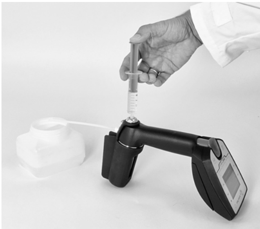
Fig. 8: Filling sample with a syringe
