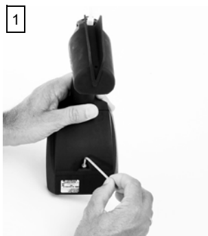
Fig. 12: Removing the battery compartment
