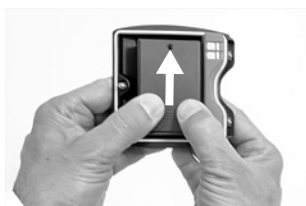
Fig. 13: Removing the cover of the battery compartment
