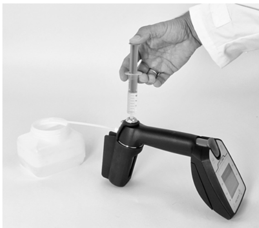
Fig. 8: Filling sample with a syringe
