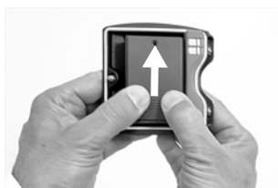
Fig. 13: Removing the cover of the battery compartment
