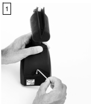
Fig. 12: Removing the battery compartment
