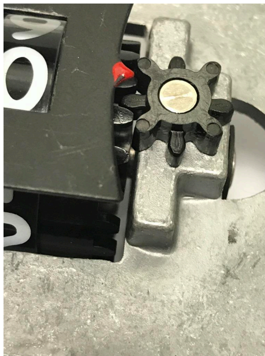
Figure 34: Pinion counter wheel alignment on whole numbers
