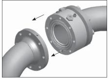
**Step 3:** Once the now-detached arm has been secured and put out of the way, remove the three (3) O-rings and two (2) O-ring spacers. Inspect and clean all machined surfaces to ensure that there are no nicks, scratches or burrs.
