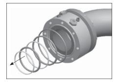
Nord-Lok<sup>™</sup> Washers – Coarser serrations must face inward and lock together
