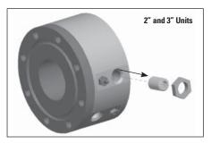
**Step 1:** Remove bearing plug bolts to access respective ball race.
