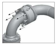
**Step 2:** Remove all split flange bolts on the side of the swivel attached to the free moving end. With the bolts loosened, support this side of the loading arm along with any other parts attached to it which might move freely when the bolts are removed. Remove bolts, starting with lowest on flange, leaving top bolts for last. Be careful not to damage sealingflange module face and bolts.
