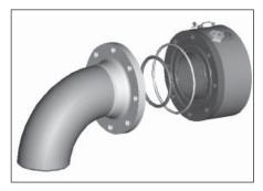
**Step 5:** Carefully align swivel tail and insert into body.
