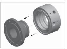
**Step 4:** Carefully remove dynamic environmental seal. Clean and inspect all machined surfaces and carefully press new environmental seal into groove. NOTE: Lube seal with light machine oil.
