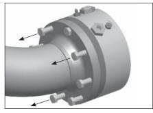
**Step 4:** With the rest of the loading arm still secured from movement, loosen the bolts on the other side of the swivel. Swivel module should fall away easily to expose environmental and O-ring seals. Secure product seal.
