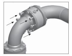
body. Set seal spacer ring inside purge seal, followed by main seal. Set SST smooth bore ring inside main seal, then cap entire seal/spacer combination with sealing flange. Torque bolts to specified value.
