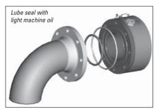
**Step 5:** Inspect and clean all machined surfaces. Press new static environmental and main seals into sealing grooves on swivel module tail.
