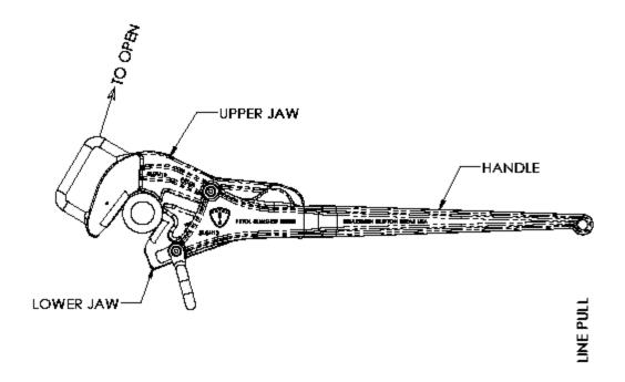
To remove the tong from the pipe, simply open the tong by pulling on the upper jaw as shown in the diagram above.
