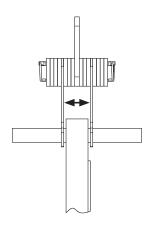
Set the width of the Flange Lifter by removing the Lynch Pins and placing the Lifting Plates between the proper number of Spacers to allow for the plates to be wider than the flange. Keep the Lifting Link centered between the Lifting Plates, and use every Spacer.
