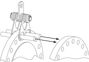
For bolted connections, guide the working flange onto its connecting flange using the flange bolts and bolt holes. Secure the working flange to the connecting flange at four separate bolt locations. Then remove the top two flange bolts and the Flange Lifter, so it is no longer lifting between the flanges. Reinsert the top two flange bolts and lift them with the Flange Lifter on the outside of the working flange while completing the connection.
