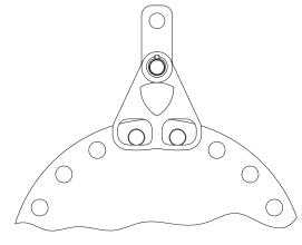
Insert two flange bolts through the Lifting Plate bolt openings and through the top two flange bolt holes. Adjust the Flange Lifter, so the flange is lifted without tilting.
